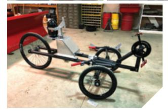
The frame supports a bracket behind the rider that holds the hydraulic reservoir, the accumulator that stores the energy and the hydraulic motor. "We were able to integrate many component mounts into the hydraulic reservoir, so we didn't require a bunch of separate brackets," says Rea. "Through doing that, we got rid of some weight and also made everything more streamlined."
