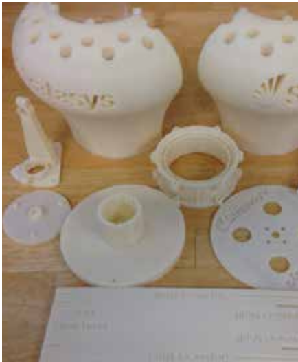
Figure 3. Parts of a Stirling engine printed with a 3D polymer printer.
