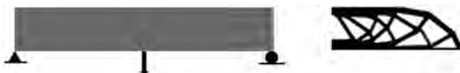
Figure 1 Topology optimization, (left) design domain and load, (right) material distribution for half of beam (Black means material and white means no material)
